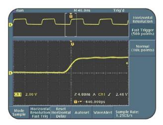
Figure 3.5: Magnified display with Fast Trigger (500 points) mode
