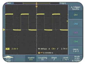
Figure 1.9: TRIGGER Section menu-based controls
