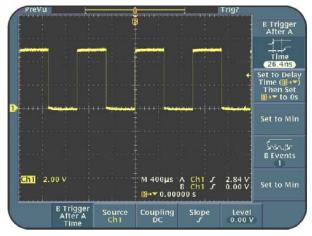
Figure 1.8: Menu-based controls for the B TRIG button
