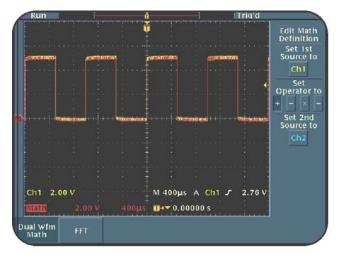
Figure 1.5: TDS3000 oscilloscope MATH men-based controls
