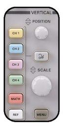
Figure 1.3: TDS3000 VERTICAL section controls
