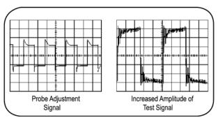
Figure 1.21: Overcompensated probe
