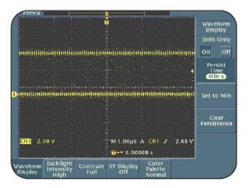
Figure 6.12: Clock signal with Dots Only On
