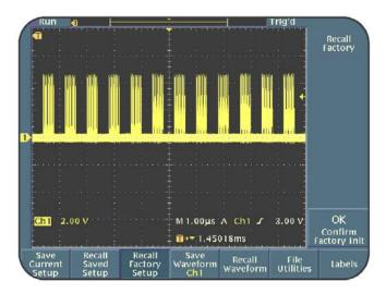
Figure 3.6: Unstable overlapping waveforms
