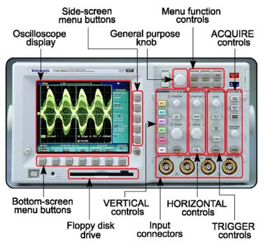
Figure 1.1: A TDS3054 digital phosphor oscilloscope
