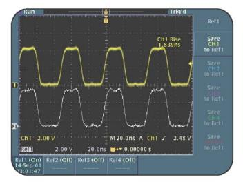
Figure 6.7: Recalled reference waveform
