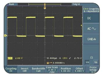
Figure 1.4: VERTICAL menu-based options for CH1
