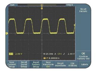
Figure 6.2: 20 MHz CLOCK signal
