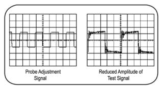
Figure 1.20: Undercompensated probe
