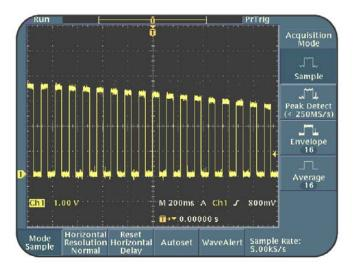
Figure 5.2: Noisy variable amplitude signal
