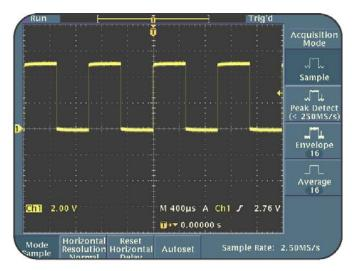
Figure 1.11: Menu-based functions for the ACQUIRE section
