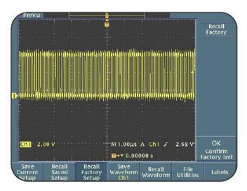
Figure 6.11: Clock signal in vector form
