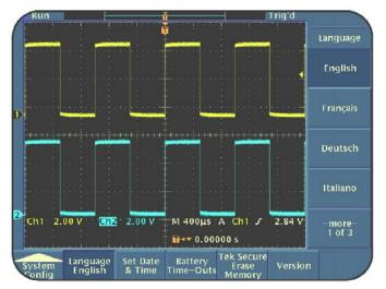
Figure 1.19: CH1 Probe Compensation Signal
