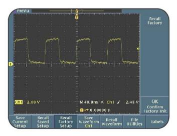
Figure 2.3: Dimmed waveform display with stopped signal acquisition and shifted waveform
