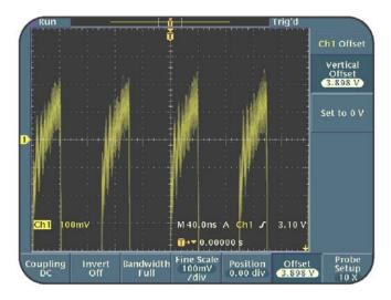
Figure 2.7:Changed vertical waveform expansion reference with respect to a waveform
