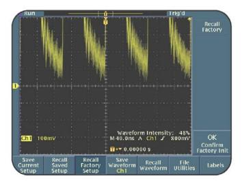
Figure 2.6: Vertically expanded waveform around the center graticule line
