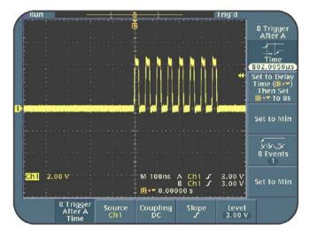
Figure 3.7: B TRIG enabled after a delay of about 800us
