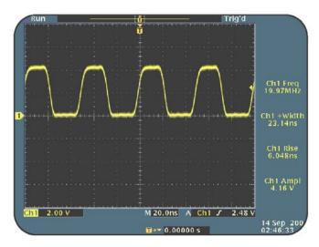
Figure 6.3: Automatic measurements
