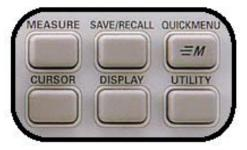
Figure 1.12: TDS3000 front panel menu function controls
