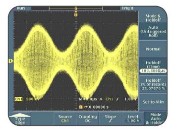
Figure 4.5: AM signal, with trigger holdoff
