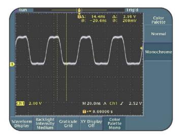
Figure 6.10: Monochrome display mode
